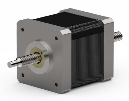
In a non-captive actuator linear actuator, the lead screw does not have an anti-rotation feature. Instead, external mechanical components separate from the motor are introduced into the design to keep the lead screw from rotating. As a result, the lead screw moves back and forth axially by restricting its rotation, which then drives the device it is attached to back and forth.
