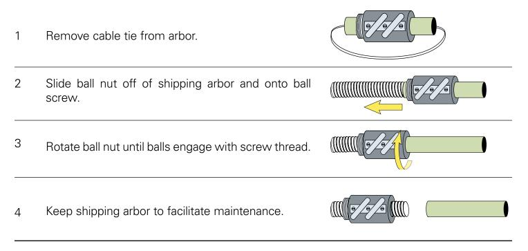
**CAUTION:** Removing the arbor without proper support will result in the loss of bearing balls, which must be replaced as a set. For additional methods, please visit helixlinear. com.
